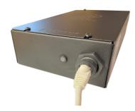
After a second or two, you should see an orange LED illuminate next to the Ethernet port.
