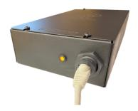
Before proceeding with the set up process, wait until the LED turns red. It will either stay solid or flash.
