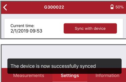
Press 'Sync with device' to synchronise your instrument's date/time setting with that of your mobile device.
