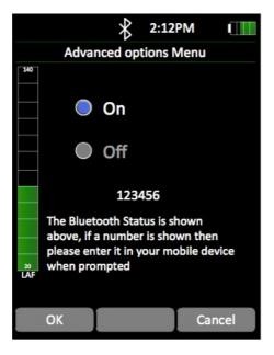
**Please note:** Bluetooth on the Optimus is connected to Port 2, meaning that it cannot be enabled as the same as GPS when used as part of an outdoor measurement kit.
