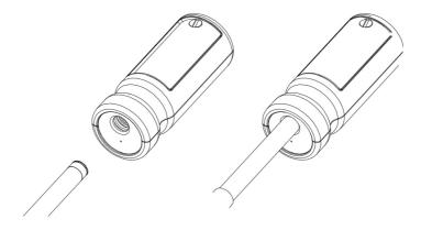
The microphone should be parallel to the body of the calibrator. Also ensure that the small bleed-hole next to the microphone cavity is not blocked as this could cause damage to the microphone.
