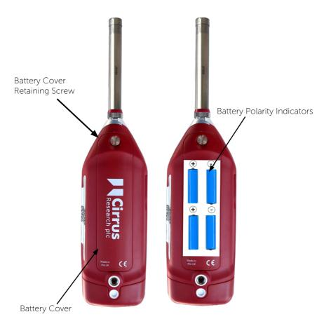
Please look carefully at the diagram inside the battery compartment that shows the correct polarity. After inserting the batteries in the correct orientation, replace the cover and tighten the locking screw.
