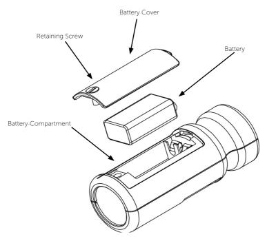
1. Unscrew the screw holding the battery cover on, using a coin or the keyring provided.
