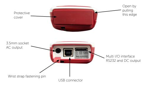
The Optimus can be powered via the multi-pin connector on the bottom of the instrument. Power can be connected using a ZL:171 Optimus power input cable (2.1 mm power jack, 2 m) or via a ZL:176 Optimus 12 V battery pack cable.
