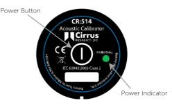
calibrator can be turned on by pressing and holding the power button for three seconds. Release the button and the indicator will flash to show that the unit is in permanent-on mode. Press the power button again to switch off the calibrator.
