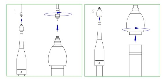
Care must be taken at this step as the diaphragm of the microphone capsule will be exposed and is easily damaged.
