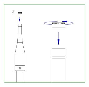
4. Connect the acoustic calibrator and select the 94dB level.
