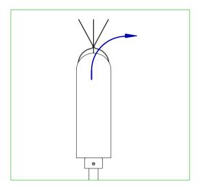
2. Carefully unscrew the electrostatic actuator unit from the microphone capsule
