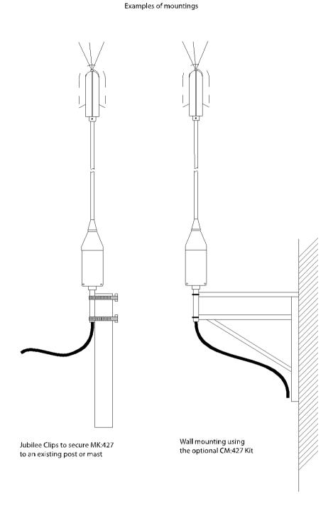
The unit is supplied with a standard mounting kit to enable the unit to be fixed to a pole or similar.
